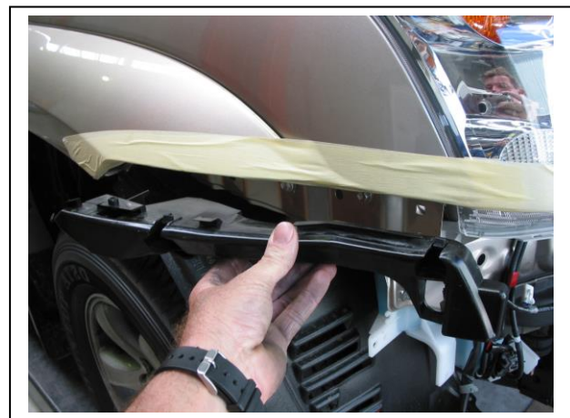
Figure 2 – Drivers side shown. Removing bumper cover clip assembly.
